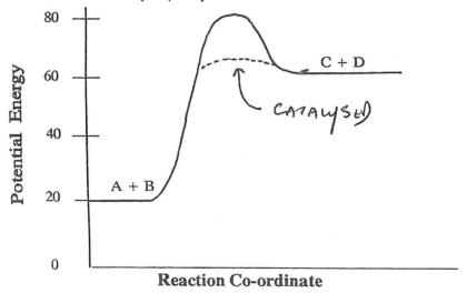
An energy profile diagram is shown above for the reaction
